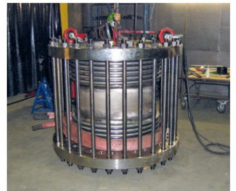
Testing a metal expansion joint with helium.
