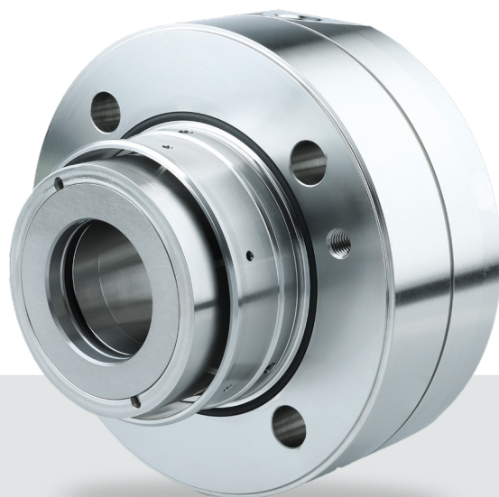
EagleBurgmann SHI mechanical seals are specially designed for very high pressures, high sliding speeds and high temperature ranges due to a loosely inserted sliding ring and other design features.
